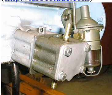
Double oil pumps. Note nipples for inlet and outlet to turbo.
