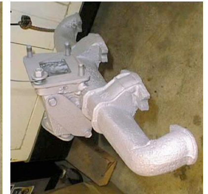
TurboStude exhaust with flange for TO-3
