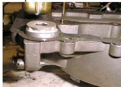
Seal on accelerator pump of AFB
